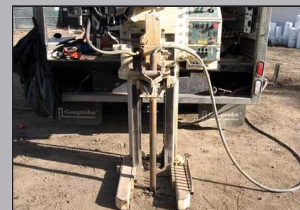
Figure 3. RegenOx Direct-Push Application
