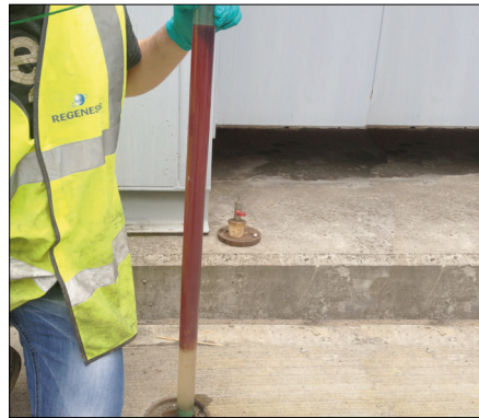
LNAPL recovery pre and post treatment
