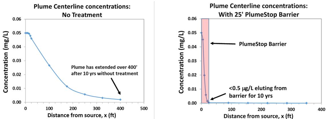
**Figure 4:** Simulated plume centerline concentration results for PFOA or PFOS. The graph on the left shows the natural migration of the plume after 10 years with no treatment, and the graph on the right demonstrates the capture longevity of a PlumeStop barrier treatment on the same plume.
