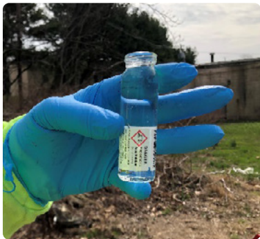
Figure 8 - Sample pulled from a PDB bag and free of suspended carbon.
