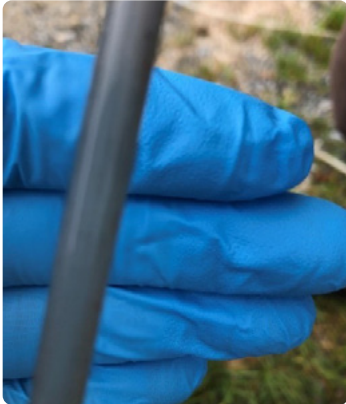
Figure 3 - Image of tubing left in well and coated with PetroFix
