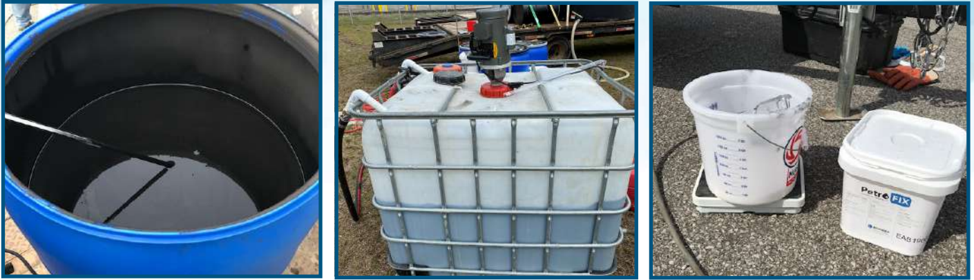
FIGURE 4 Image on left shows undiluted PetroFix in a drum prior to homogenization. PetroFix doesn't fully fill the drum and this is normal (a 400 lb drum of PetroFix contains approximately 41 gallons of product). The image in the middle shows an example transfer and PetroFix mixing setup where a 330-gallon tote was chosen as the mix tank. The picture on the right shows some PetroFix electron acceptor being weighed before placement into the mixing tank.
