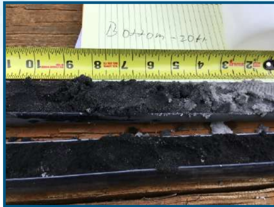
FIGURE 8 Photo showing an in-field verification of PetroFix distribution and its optimal coverage. Gray soil in upper right shows the edge of the injection zone where PetroFix not injected.
