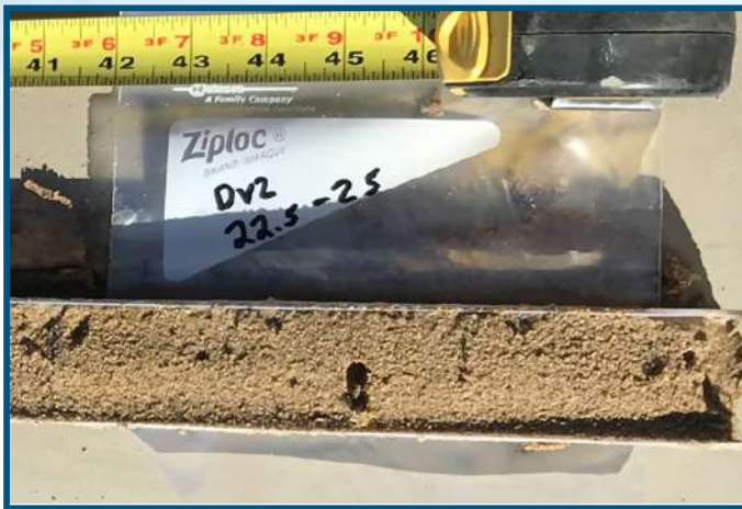
FIGURE 1 The photo on the left shows a soil core collected before a PetroFix application. The photo on the right shows a soil core collected after a PetroFix application exhibiting black soil where the PetroFix was successfully distributed.
