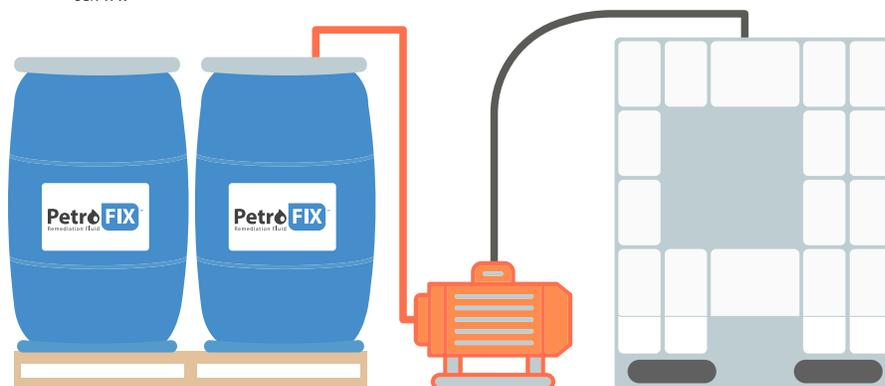
The image shows an example PetroFix transfer and mixing setup where a tote was chosen as the mix tank
