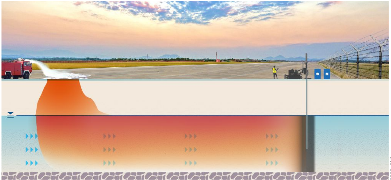
A graphic depicts a PFAS plume in groundwater due to a fire-training exercise as well as the application of a colloidal activated carbon (CAC) barrier at a downgradient plume boundary to effectively contain the plume from moving offsite.
