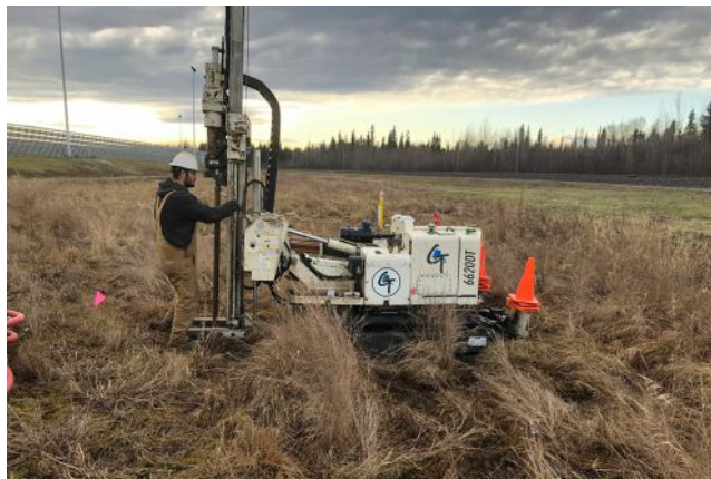
REGENESIS Remediation Services mix and monitor remedial amendments in a services trailer onsite (top). Then the remedial amendments are placed in situ using a GeoProbe (bottom).
