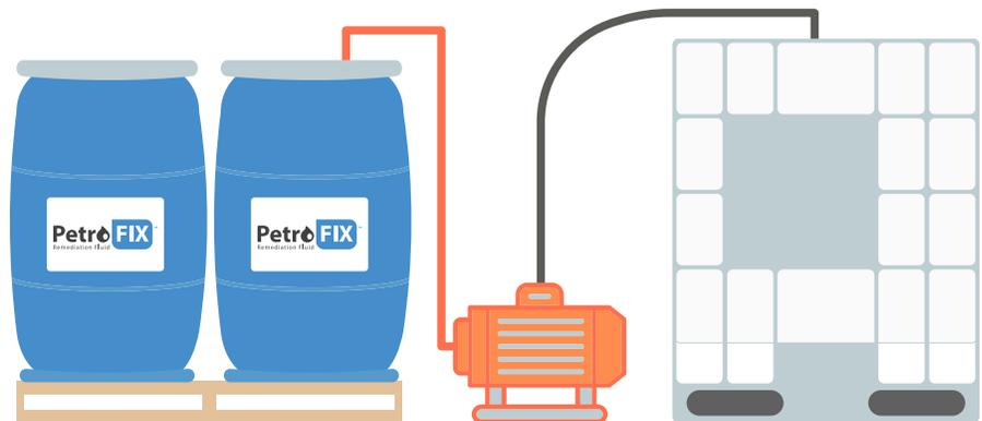
The image shows an example PetroFix transfer and mixing setup where a 330-gallon tote was chosen as the mix tank
