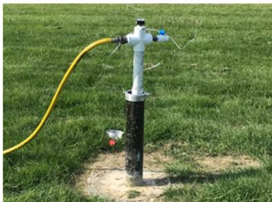
*Example of an injection head assembly mounted to an above ground well.*
