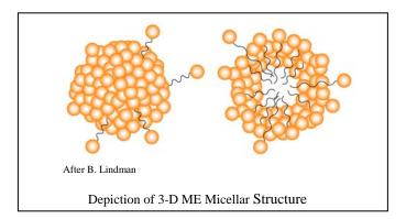
The size of the 3DMe micelles formed is very small, on the order of .02 to .05 microns in diameter. These will spontaneously form in aquifer waters when the CMC is exceeded. Thus,
