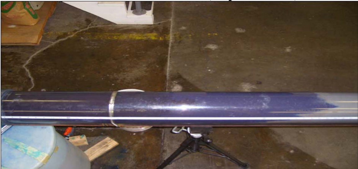
Figure 2 3DMe Movement at 13 hours (3.5 pore volumes)
