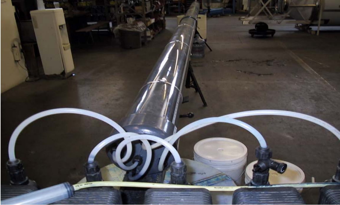
Figure 1 Experimental Packed Column (20-foot-long, 6-inch diameter)
