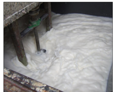
Fig.3 - 3DMe emulsion mixed with water prior to application
