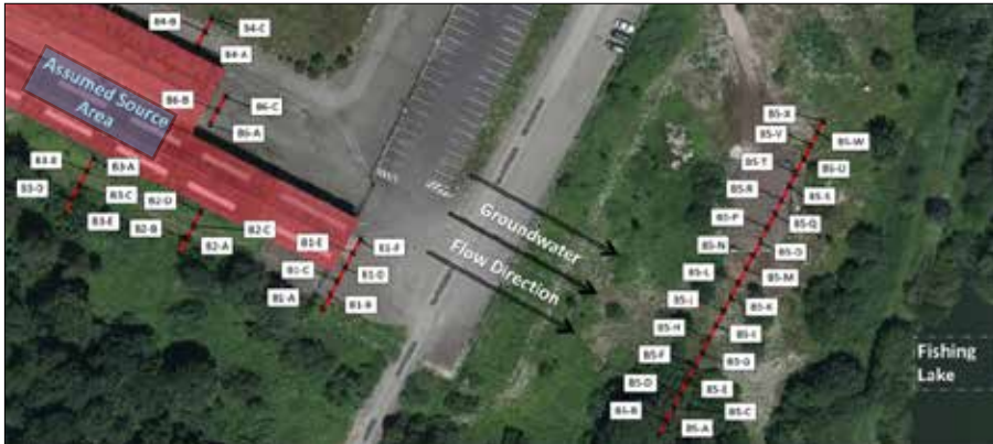
Fig. 6 Treatment zones ('barrier') locations
