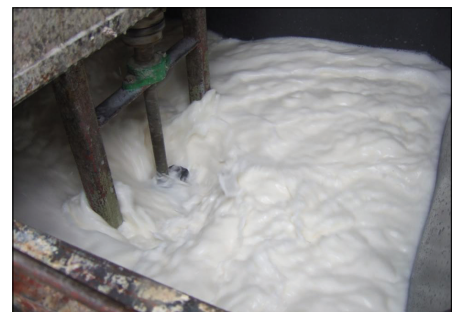
Figure 1 Mixing tank with 3-D Microemulsion
