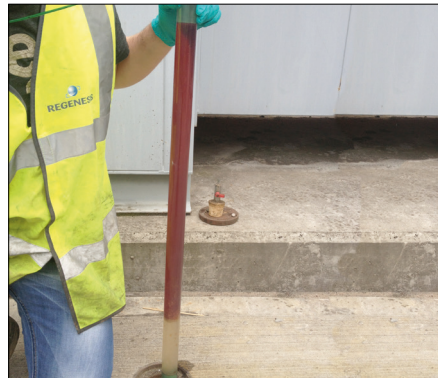
LNAPL recovery pre and post treatment
