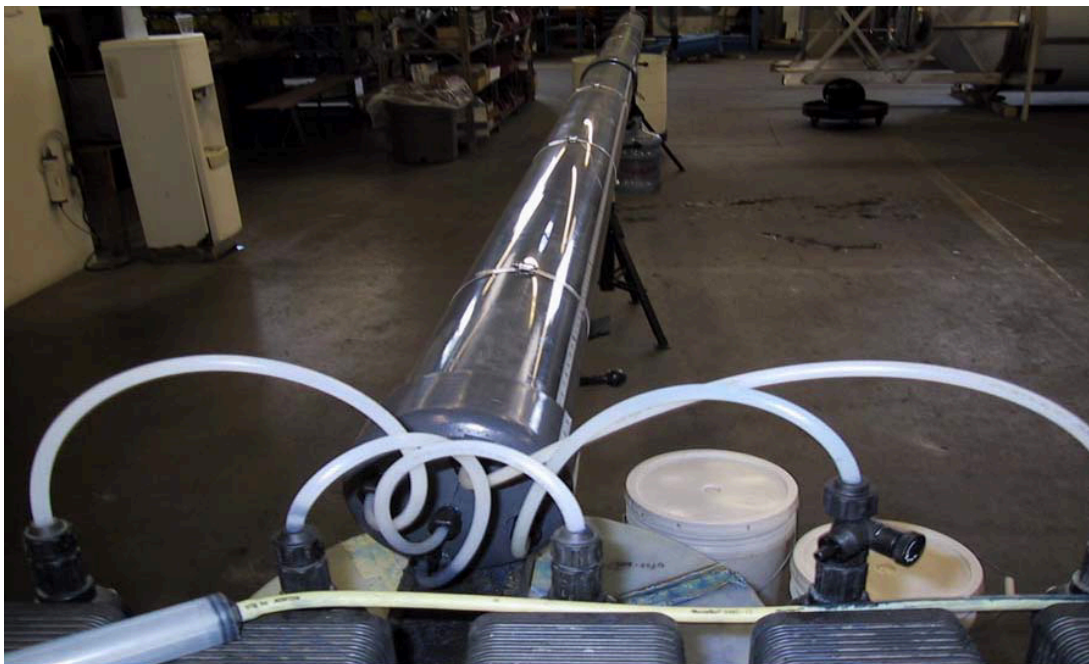
Figure 1: Packed Experimental Column (20ft long x 6in ID)
