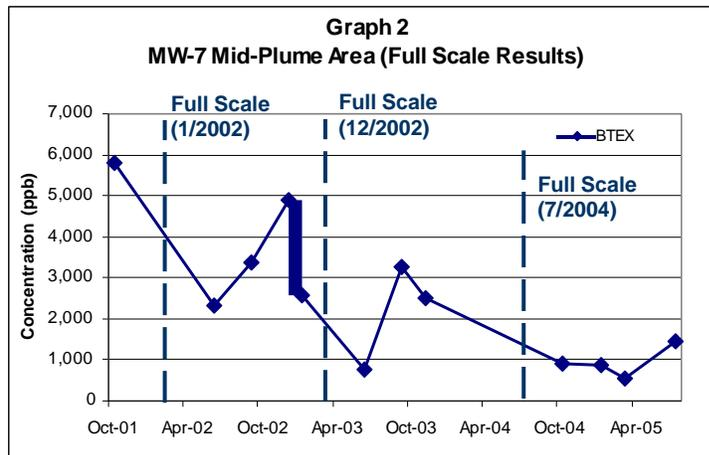
A continuous decrease in BTEX resulted in an overall contaminant mass reduction of 85%. The multiple ORC applications were successful at sustaining an aerobic environment to facilitate bioremediation within the plume.
