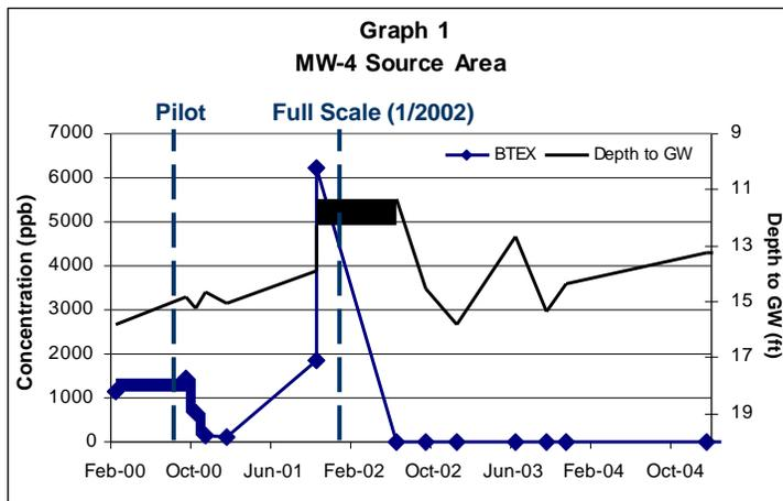
A high groundwater event resulted in re-contamination of the aquifer due to significant smear zone contamination near MW-4. October 2001 shows an increase in BTEX by more than 4,300 ppb. The full scale application in January 2002 reduced concentrations to non-detect.
