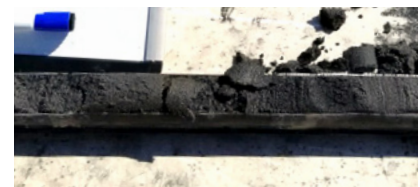
Post-injection soil core shows PetroFix distribution within the target treatment interval.
