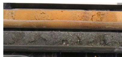
Post-injection soil core shows PetroFix distribution within the target treatment interval.
