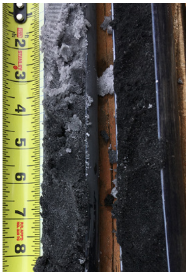
Post-injection core samples like these were taken within the treatment area to identify the depth and extent of PlumeStop applications
