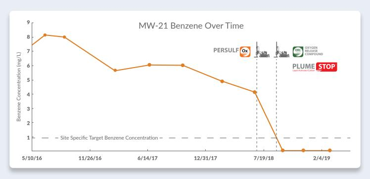
Graphs chart benzene contaminant levels, pH, Oxidation Reduction Potential and Dissolved Oxygen levels present in MW-21 pre- and post-application. The site was granted closure following two quarters of post-application monitoring.
