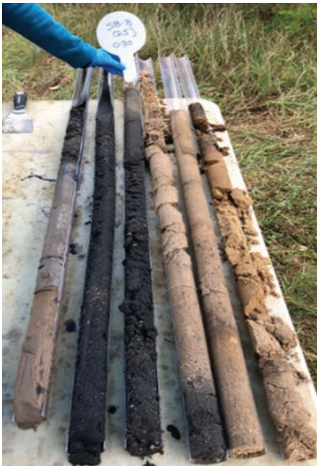
An extracted soil core showing CAC coating of soils following PRB application. The target application interval spanned the depths of the soil cores at second and third from left.
