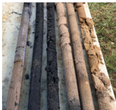
Core samples and settling tubes taken from SB8-2.5 depicting consistent PlumeStop saturation from 15-27 feet bgs.
