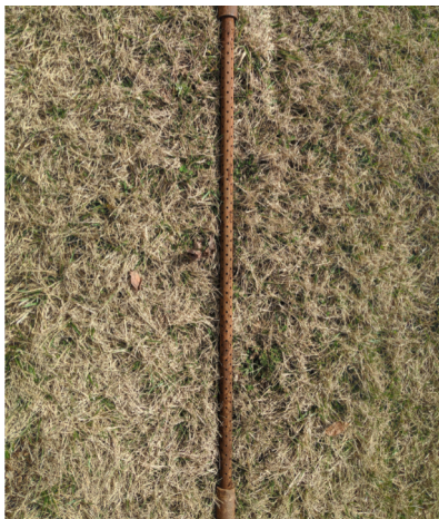
3-foot deployable multi-port injection screen used to apply PetroFix
