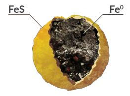
**Figure 1.** S-MicroZVI consists of ZVI particles that are coated with iron sulfide.
