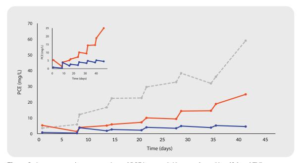
**Figure 2.** Aqueous sample concentrations of PCE in control **Untreated --- Unsulfidated ZVI —— S-MicroZVI** — The inset graph shows the same data zoomed in to better illustrate the difference in reactivity between unsulfidated ZVI and S-MicroZVI.
