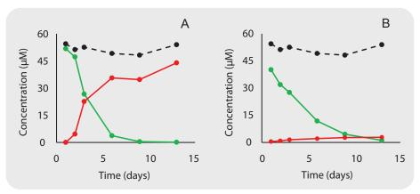
**Figure 3.** Aqueous concentrations of chlorinated ethanes in samples treated with A) unsulfidated ZVI and B) S-MicroZVI. **1,1,1-TCA control (no ZVI)** ---
