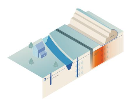
Figure depicting an in situ colloidal activated carbon permeable reactive barrier preventing migration of PFAS to sensitive receptors.
