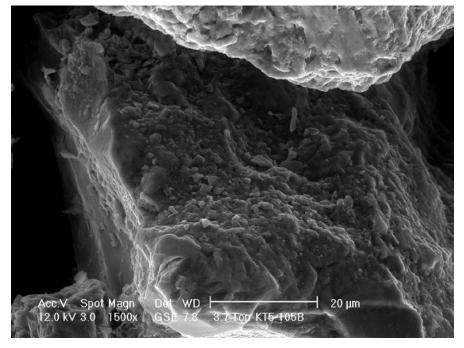
Micro-scale image showing CAC coating individual sand grains.
