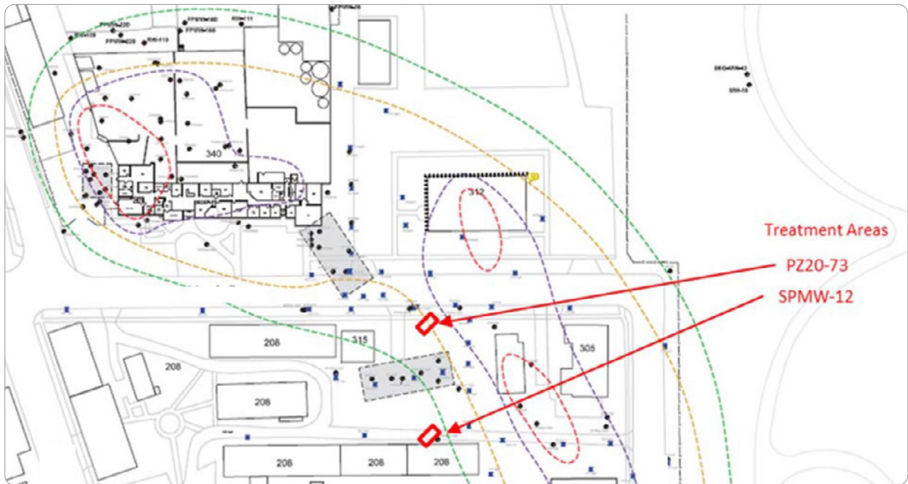
Pilot test treatment areas shown relative to the chlorinated solvent plume.
