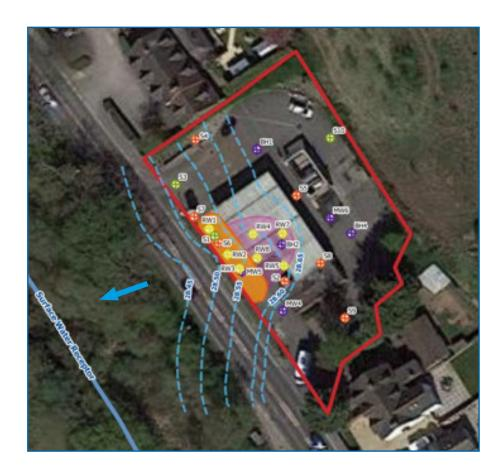
Fig. 1 Plan view showing the contaminant plume (purple) , PetroFix IPRB (orange) and groundwater direction (blue) ©SLR Consulting
