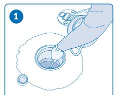
Measure and record the depth to groundwater and the total depth of the monitoring well on the Chain of Custody form.
