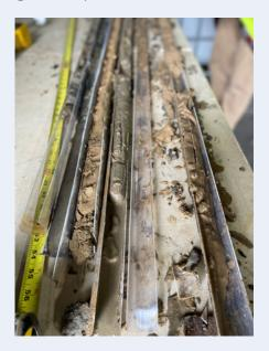
Prior to the *in situ* injection treatment, REGENESIS completed design verification testing (DVT) to confirm the target treatment zone (TTZ) and other design parameters. As part of the DVT, a clear water injection test was performed to confirm the feasibility of injecting the design volume and to ensure PlumeStop coverage throughout the barrier. Continuous soil cores were also collected over the target treatment interval (i.e., 5 to 30 feet bgs).
