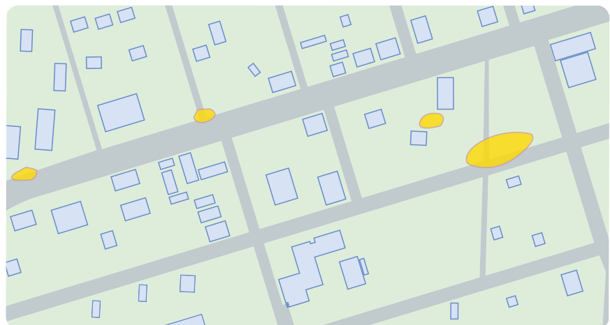
Vestiges of the PCE plume post-application. No concentrations remain above the Residential Vapor Exposure Groundwater Screening Level for PCE.
