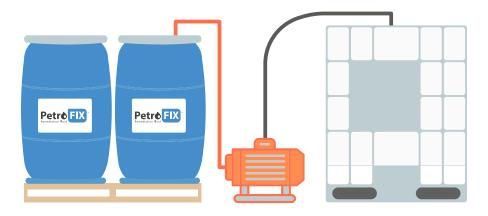
The image shows an example PetroFix transfer and mixing setup where a 330-gallon tote was chosen as the mix tank
