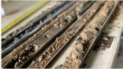
Soil cores collected as part of design verification testing
