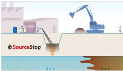
SourceStop Liquid formula is applied to soils at the base of an excavation as a horizontal barrier layer to prevent PFAS leaching.
