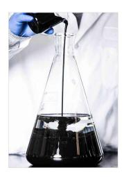
SourceStop can be poured into wells or injected directly into the capillary fringe and the groundwater under source areas, where it easily disperses within contaminated aquifer materials. This is unlike powdered activated carbon (PAC) products of larger particle size which require high-pressure injection (fracking) for emplacement and do not disperse. Once in place, SourceStop rapidly sorbs contaminants, restricting their leaching from unsaturated soils and immobilize them in aquifers.
