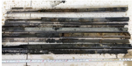
Soil cores collected during the application process depict complete coverage of PlumeStop® onto aquifer soil materials.
