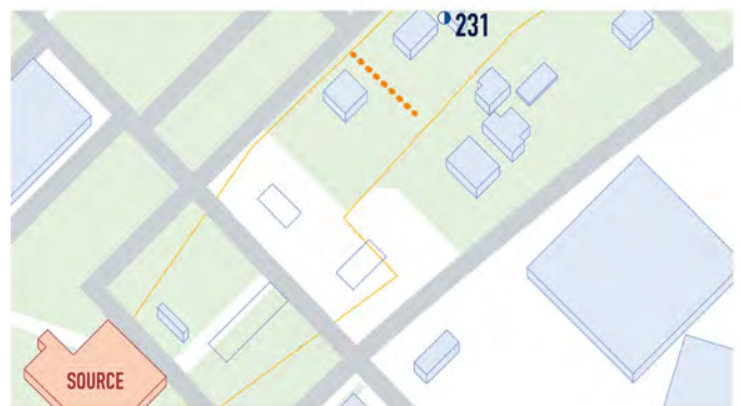
Well #231 - Approximately 120 feet away from the nearest upgradient treatment line
