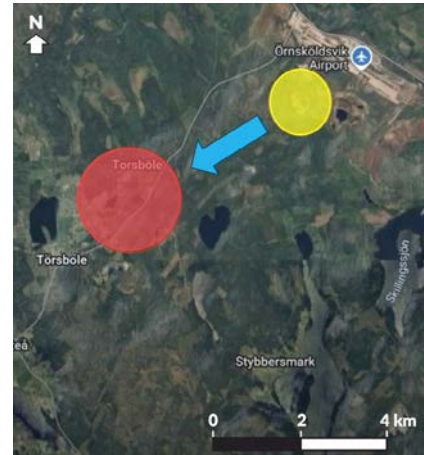
Figure 1 (above) Regional satellite imagery map showing site location. Yellow circle indicates the firefighting training area. Red circle indicates surface water locations where PFAS have been detected. Blue arrow indicates groundwater flow direction. Figure provided by Sheeba Environmental and updated by REGENESIS.
